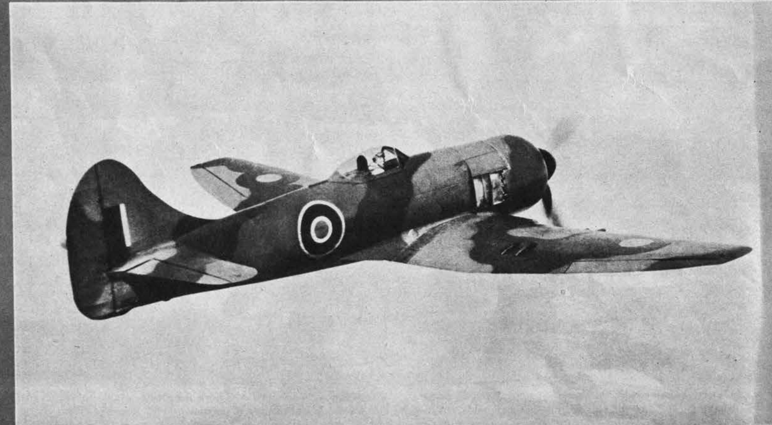
RUDDER EXTENSION BELOW THE BELLY LINE AND THE BIG FIN'S FORWARD FAIRING CURVE CHARACTERIZE TAIL ASSEMBLY OF BOTH TEMPEST II AND V
